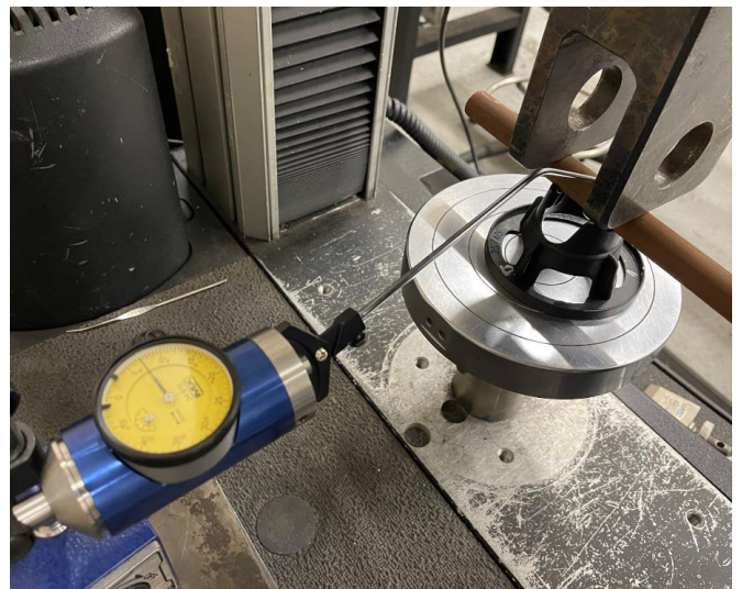
Fig 2: Showing deflection measurement under load.
