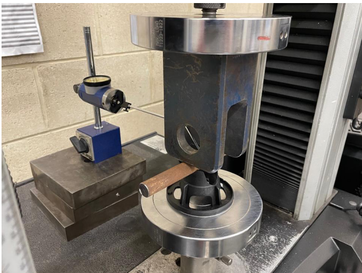
Fig 1: Showing load test / deflection set up.
